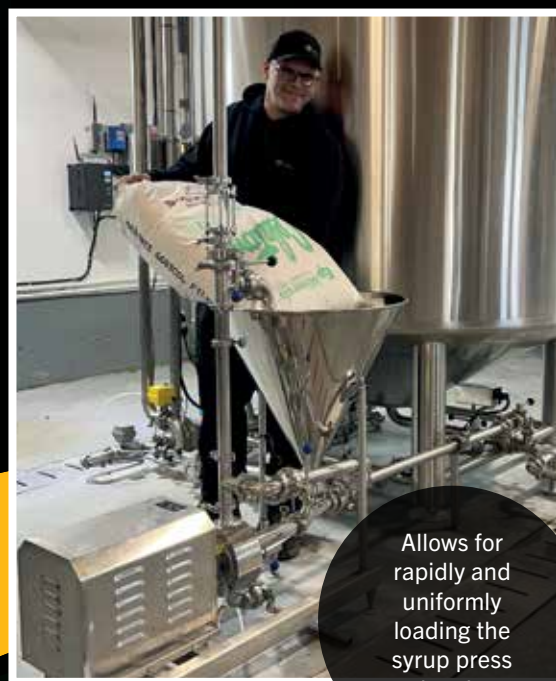
Dynamic Mixer YRL 1-100 with 5.5 HP motor 668429
