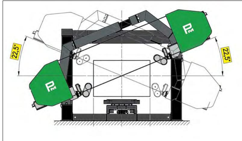
**New diamond wire profiling plant, equipped with CNC system, 7 axes controlled for wire inclination up to 22.5°.**
