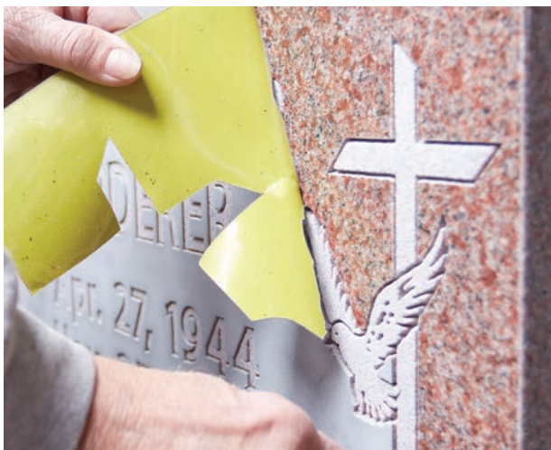
Remove Stencil: Stencil removes cleanly in one piece.
