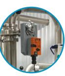
The vacuum protection valve safely prevents sap overflow in your moisture trap or your vacuum pump without shutting vacuum down.
