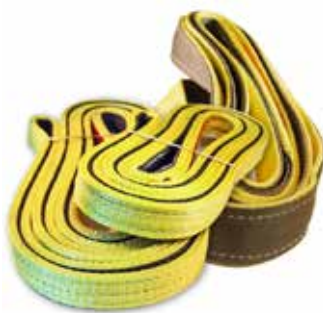
1" and 2" Straps with Cordura Straps have a cordura wear strip sewn around the inside to decrease wear and give the strap extra grip on surfaces.
