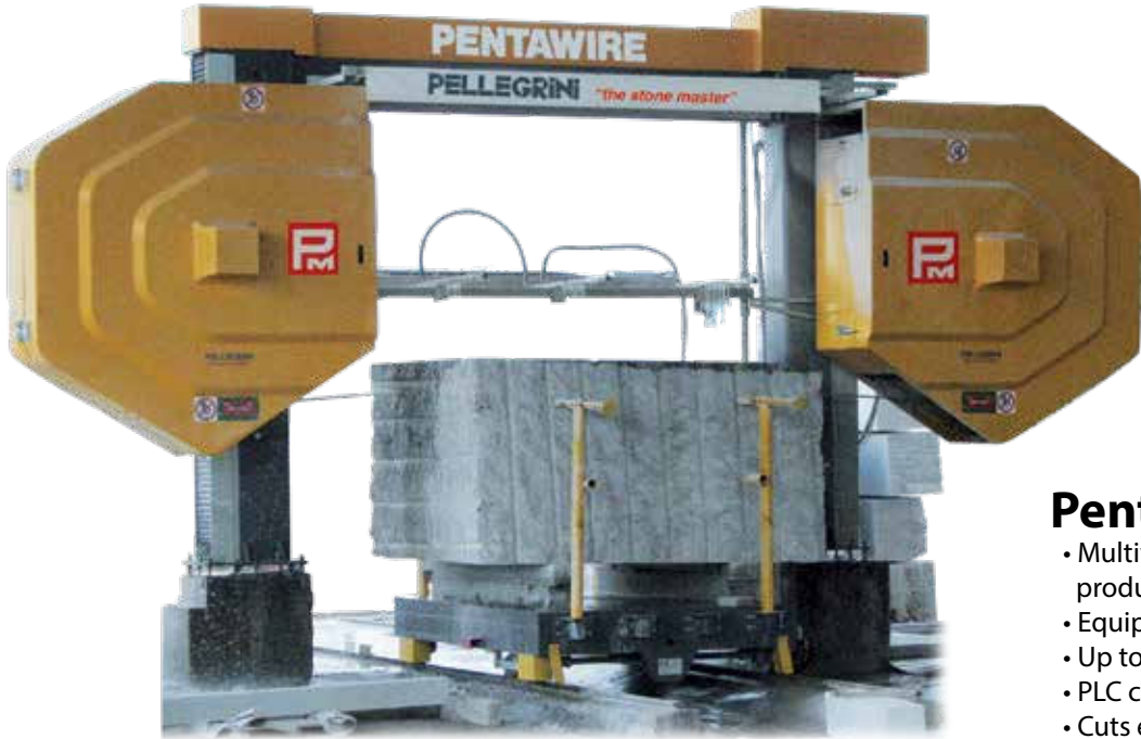
Patented "Multipull" bearings for independent tensioning of each wire.
